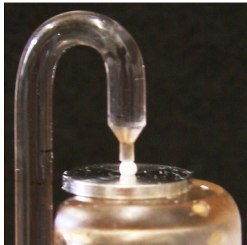
Fig. 6. TMA sample holder designed to measure the film's glass transition temperature in situ.
